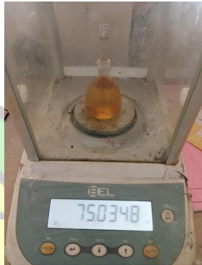
**Gambar 16** Penimbangan piknometer berisi biodiesel
