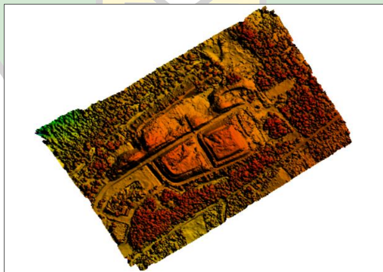
Gambar 2.8 Digital Surface Model (DSM) (Sumber: Software Agisoft Metashape, 2023)
