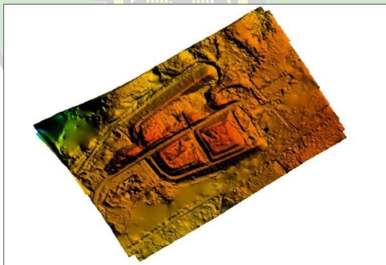
Gambar 2.9 Digital Terrain Model (DTM) (Sumber: Software Agisoft Metashape, 2023)
