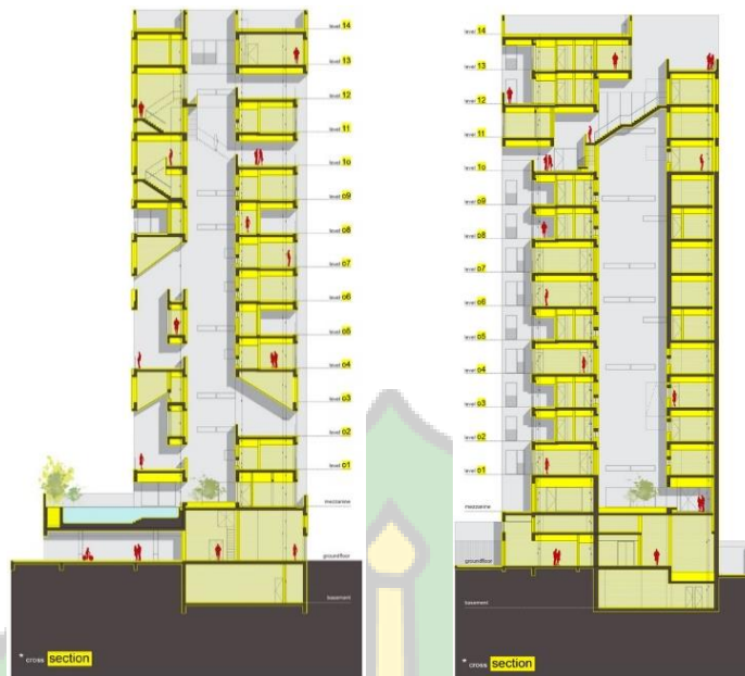
Gambar 3. 10 Potongan Wafra Wind Tower
