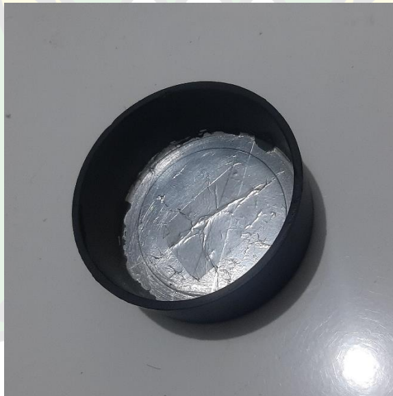
Gambar 3. 5 Tutup pipa dilapisi aluminium foil
