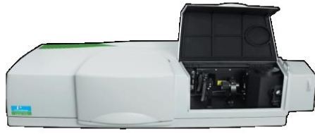
Gambar II.8 Alat spektrofotometer UV-Vis Sumber: ( https://resources.perkinelmer.com )
