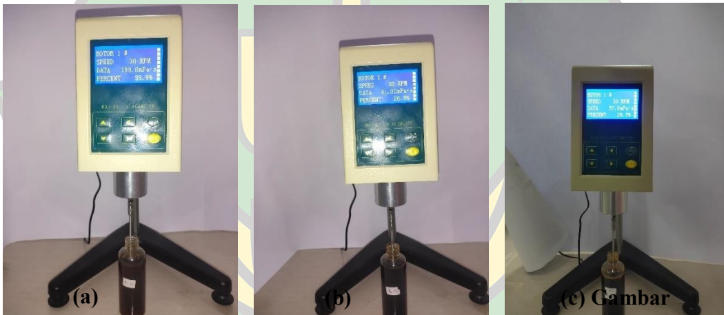
(a) (b) (c) Gambar V.12 Hasil uji viskositas, (a) formulasi 1, (b) formulasi 2, (c) formulasi 3
