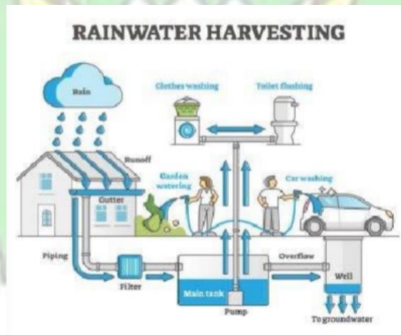
Gambar 5.50 Skema Sistem Jaringan Rainwater Harvesting (Sumber: Depositphotos)
