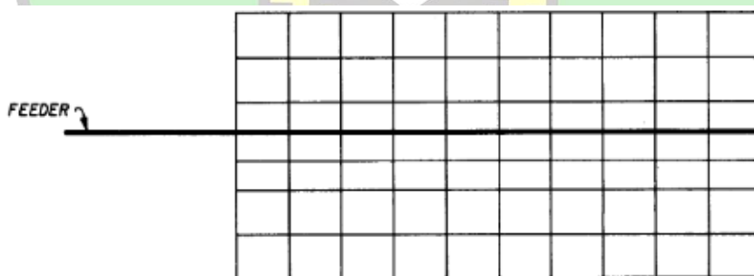
Gambar 2.3. Pipa Distribusi Sistem Grid Iron
