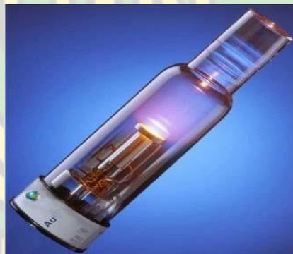
Gambar 2.9. Lampu Katoda Berongga ( Hallow Cathode Lamp ) (Sumber : http://mc-tester.com/lampu-katode-berongga-hollow-cathode-lamp-series-aas-atom/ )
