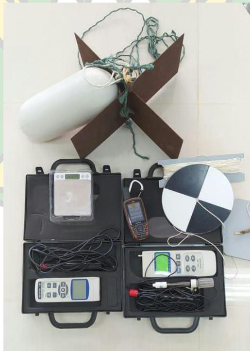
*Thermometer, Floating draught, secchi disk, DO meter (Dissolved Oxygen Meter, timbangan digital dan GPS*
