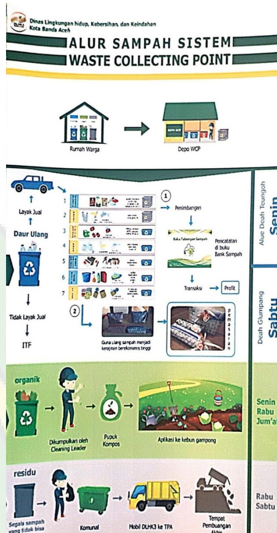
Gambar 2. Alur Sampah Sistem Waste Collecting Point (WCP)
