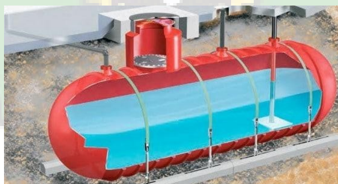
Gambar 4.17 Ground Water tank .
