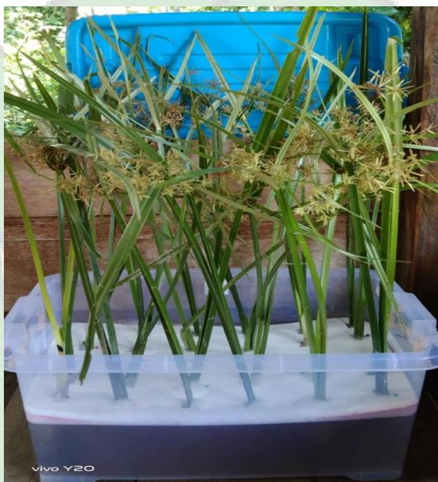
**Gambar 3.3** Reaktor *Constructed Wetland*
