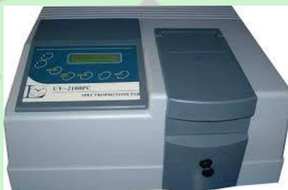
**Gambar 3.8** Alat spektrofotometri UV-VIS
