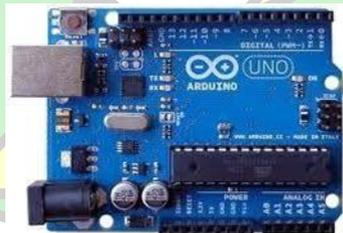
Gambar 2.7. Board Arduino
