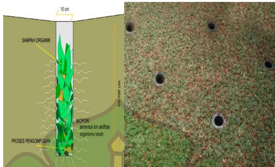
Gambar 4. 21Sumur Biopori
