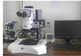
Gambar 3.19 Mikroskop stereo binokuler
