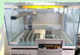
Gambar 3.24 Alat spektrometer XRF (X-Ray Fluorescence)
