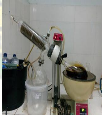
Proses vacuum rotary evaporator
