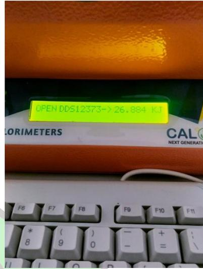
**Gambar 10.** Bom kalorimeter
