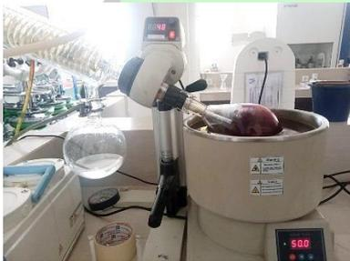
**Gambar 3** Proses evaporator
