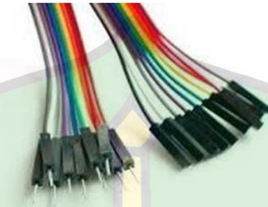
Gambar 2.10 Kabel Jumper
