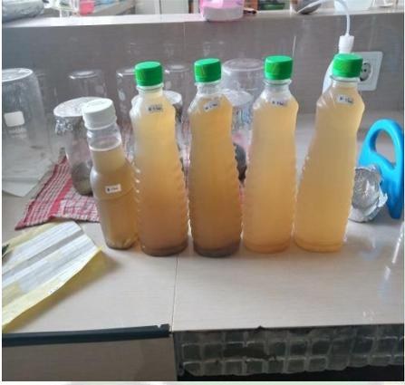
A photograph showing five clear plastic bottles with green caps, each containing a yellowish liquid. They are arranged on a white lab bench. In the background, there are various lab glassware and a blue pair of scissors.            | Sampel limbah cair RPA setelah perlakuan pada reaktor <i>biosand</i> filter                     |
