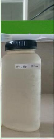
A photograph of a single white plastic bottle with a black cap. The bottle is filled with a white, opaque liquid. A small label is attached to the bottle.                                                                             | Sampel limbah cair RPA setelah perlakuan kombinasi aerasi terdifikasi dan <i>biosand</i> filter |
