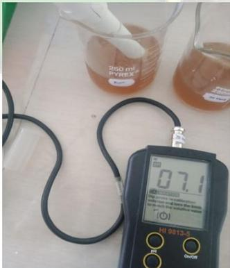
A photograph showing a digital pH meter (HI 9913-5) with a black probe inserted into a beaker containing a yellowish liquid. Another beaker with a similar liquid is visible next to it. The meter's display shows a reading of 07.1. | Pengukuran pH                                                                                   |
