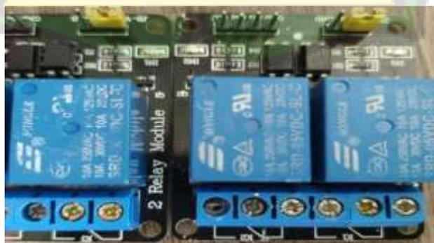
**Gambar 2.5** Module Relay
