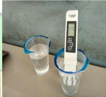
Gambar 3.5 Pengukuran Dengan Tester Air (Ph Meter) Dan Tester TSD & EC (Hold)
