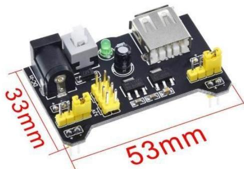
**Gambar II.10** *Breadboard Power Supply* MB102 (Chuzaini, 2022)
