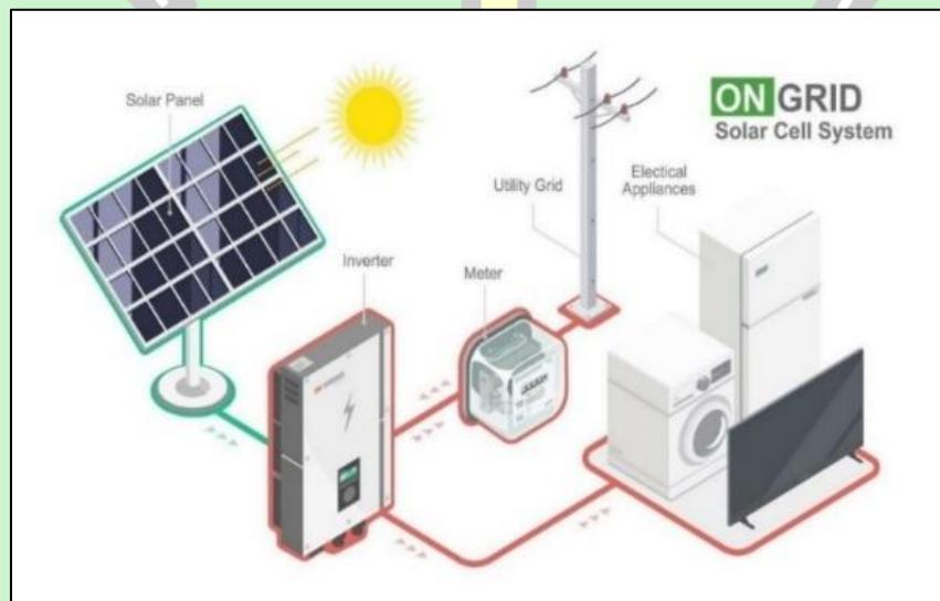
Gambar 2. 8 Sistem PLTS *On-Grid*<sup>37</sup>
