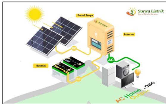
Gambar 2. 9 Sistem PLTS *Off-Grid*<sup>38</sup>
