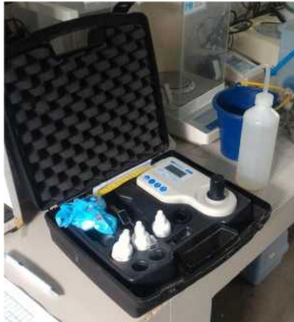
Gambar 4.17 Alat Turbidimeter di Laboratorium PDAM Tirta Daroy
