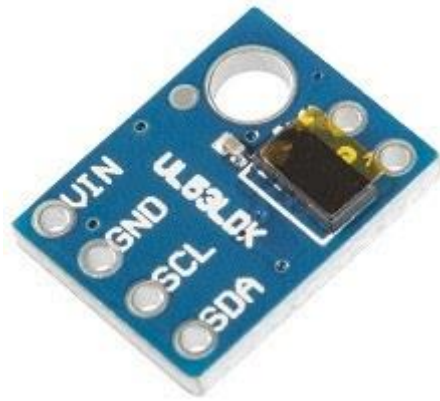
Gambar 2. 3 Sensor ToF VL53L0X (GY530)
