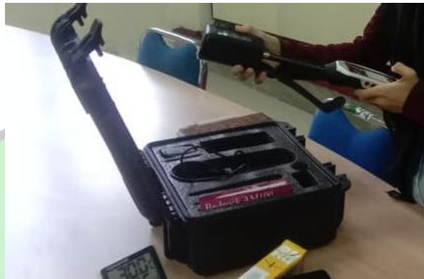
Gambar 3.11 Proses kalibrasi Sound Level Meter
