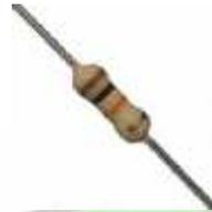
Gambar 2. 10 Resistor 10 K
