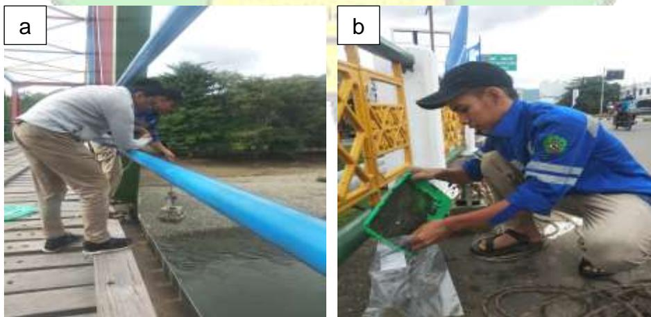
**Gambar 3.4** (a) *Sediment Grab* diturunkan, (b) Sampel sedimen dikemas
