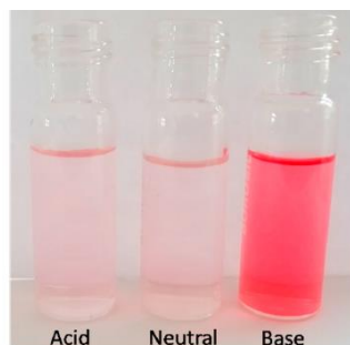
Fig. 4. Effect of pH for the coloration of Pb(II) with extract.
