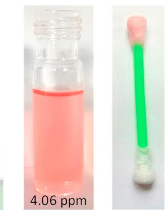
Fig. 16. Detection of Pb(II) on industrial effluent using (a) extract and (b) extract coated ear bud.
