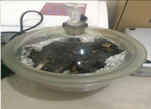
A glass desiccator with a lid is shown. Inside, a piece of banana skin is placed on a white surface. The desiccator is on a light-colored surface.                                                                |  |
