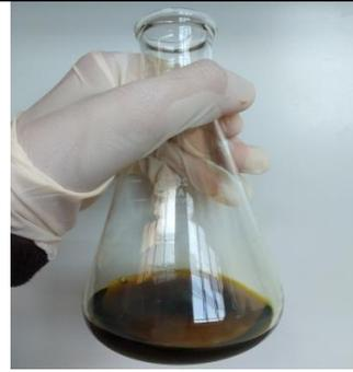
6. Ditambah 30 ml campuran  $\text{CH}_3\text{COOH}:\text{CHCl}_3$  (3:1)
