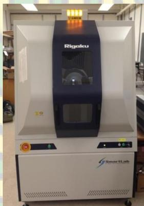
**Gambar 3.10** Alat *X-Ray Diffraction*
