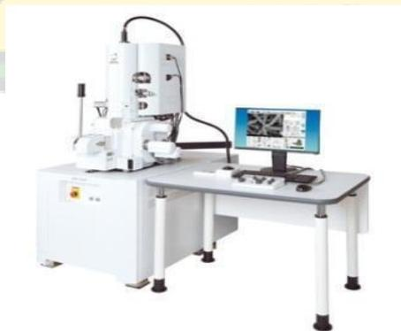
**Gambar 2.5** *Scanning Electron Microscopy* (SEM).
