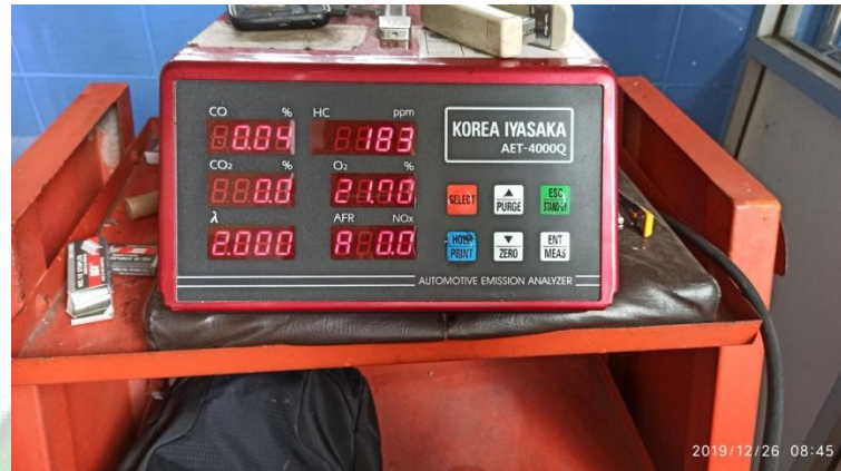
Gambar 3.4 Instrument Gas Analyzer Tester (sumber : www.kiyasaka.co.kr )
