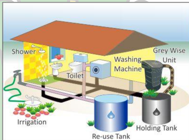
Gambar 5. 14 Sistem Grey Water Sumber : http://www.wisewatersolutions.com.au/ A R - R A N I R Y
