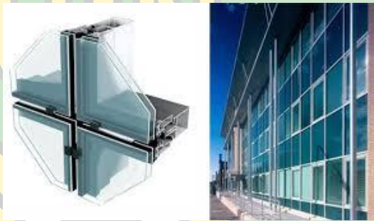
Gambar 3.8 Detail Curtain Wall
