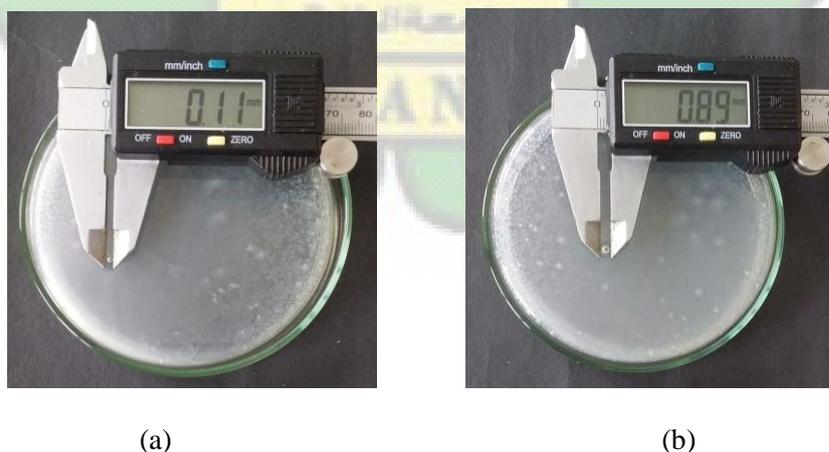
Gambar 4.5 Pengukuran Koloni Bakteri Dari Isolat Bakteri Asal Rhizosfer Mangrove, (a) SPB 1; (b) SPB7
