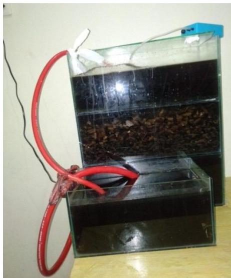
**Gambar 4.3** Proses Pengolahan *Trickling Filter*
