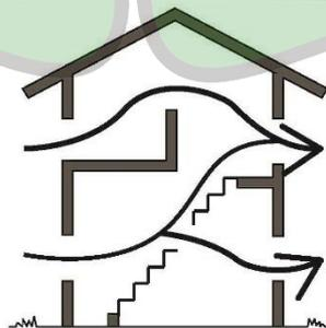
Gambar 4.42 Sistem *Cross Ventilation*
