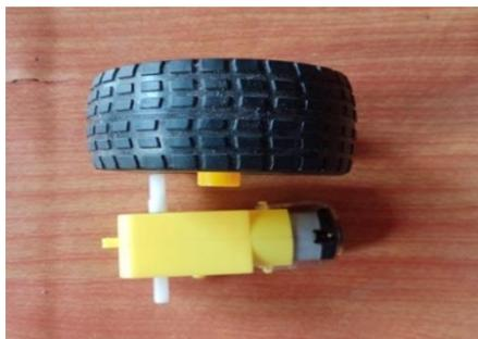
Gambar 2.6 : Motor DC Gear Box
