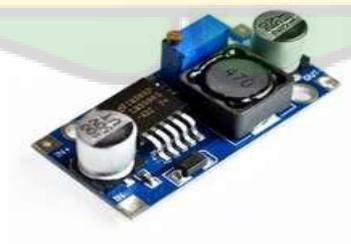
Gambar 2.7 : *Module Step Down DC*
