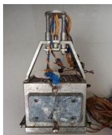
Gambar 3.3. Alat Sediment Grab
