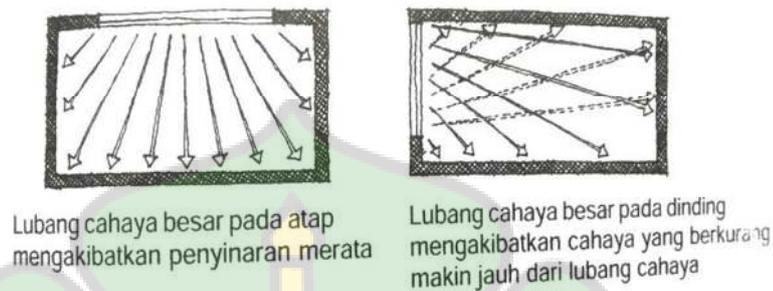
Gambar 3. 3 Lubang Cahaya Pada Atap Dan Dinding
