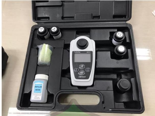
Gambar 12 *Turbidity meter* AMT21 AMTAST
