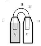
Fig.-4: A Simplified Model of the Siphon-Modified Decomposer, A = Decomposer Cylinder; B = Siphon-Like Connector; C = Aeration Cylinder 1256
