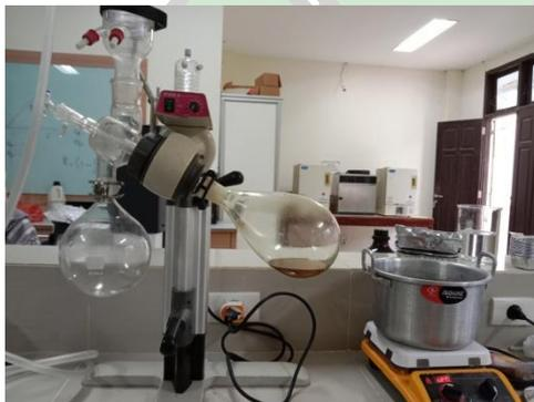
*Rotary evaporator*: alat pemekatan filtrat
