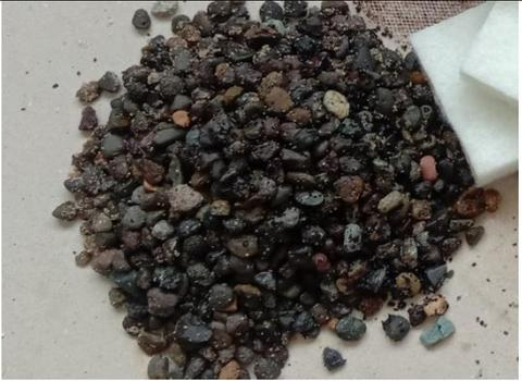
A photograph showing a pile of dark, irregularly shaped gravel filter media on a surface. | Kerikil media filter saringan bertingkat      |
