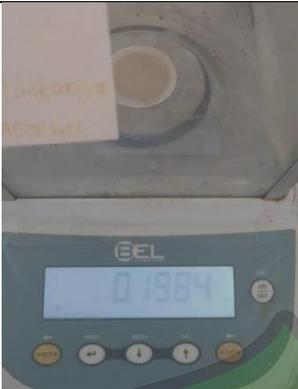
A digital scale with a blue display showing 0.1984. A piece of white paper with orange text is placed on the scale's weighing pan.                                                           | Berat kertas saring + residu kering sampel dengan massa biokoagulan 2 gram |
