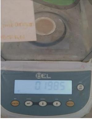
A digital scale with a blue display showing 0.1985. A piece of white paper with orange text is placed on the scale's weighing pan.                                                         | Berat kertas saring + residu kering sampel dengan massa biokoagulan 5 gram |
