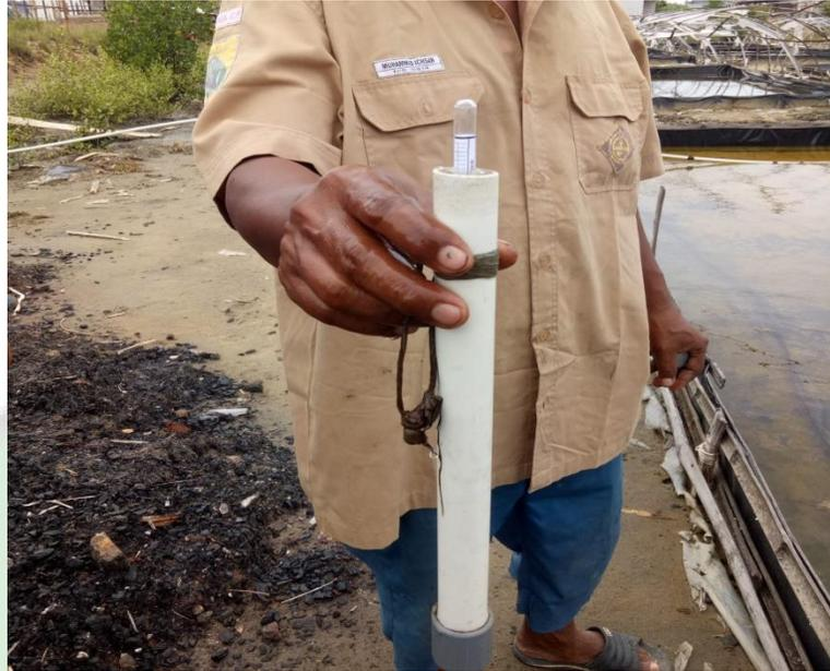
Gambar 5.19: alat mengukur takaran air garam
